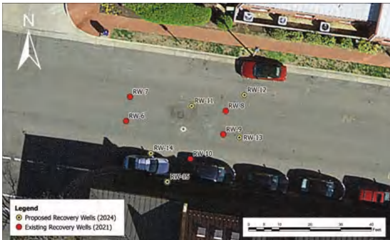
Figure 3 - Proposed Locations of New NAPL Recovery Wells
